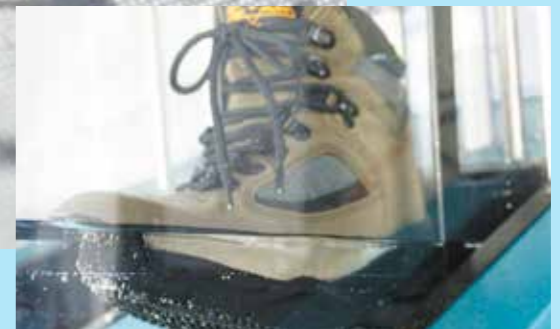
Waterproof testing of shoes by immersing a shoe in the water and simulating walking behaviors.
