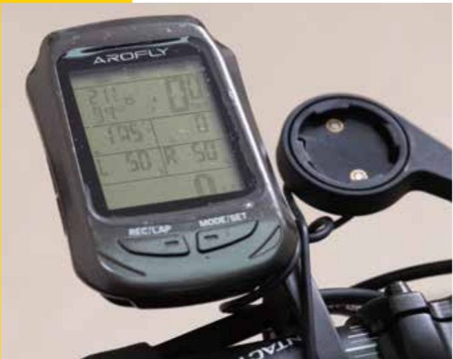
(Left) AROFLY's bike computer. Receives data from the sensor via Bluetooth. (Right) The sensor can fit both Schrader and presta valve caps which are used on the vast majority of bike tires. With no precedent for valve cap mounted devices in existence, development truly started from zero.
