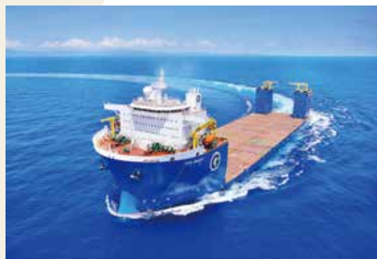
65,000 DWT Semi-submersible Deck Cargo/Heavy Lift Carrier
